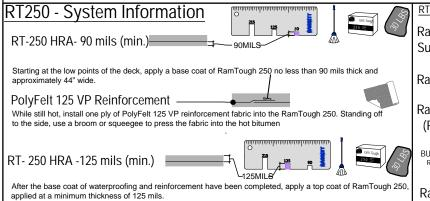
CONCRETE DECKS MUST BE MADE REASONABLE SMOOTH, DRY, FREE OF DIRT, LAITANCE, CURING
