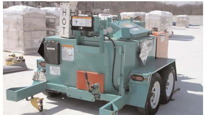
Melter must be free of foreign materials. Begin melter warm-up early enough to have hot fluid material when the work is schedule to start. Cold weather start-up will take longer. Ignite
